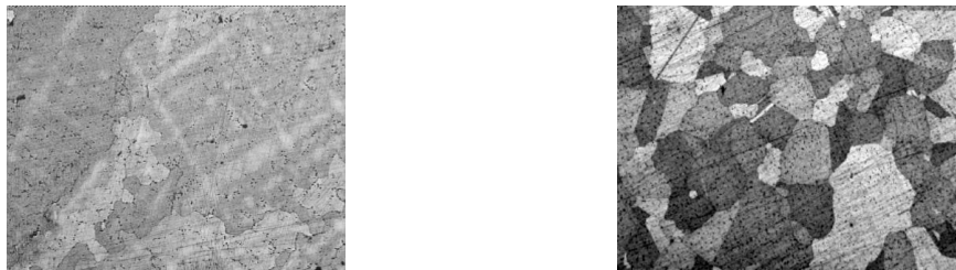
Fig. 1. Macrostructure of the GS3 nickel alloy, x100 a: before the modification; b: after the modification
