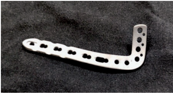
Fig. 1. A metal plate with a BG-based coating deposited on the contact surface
