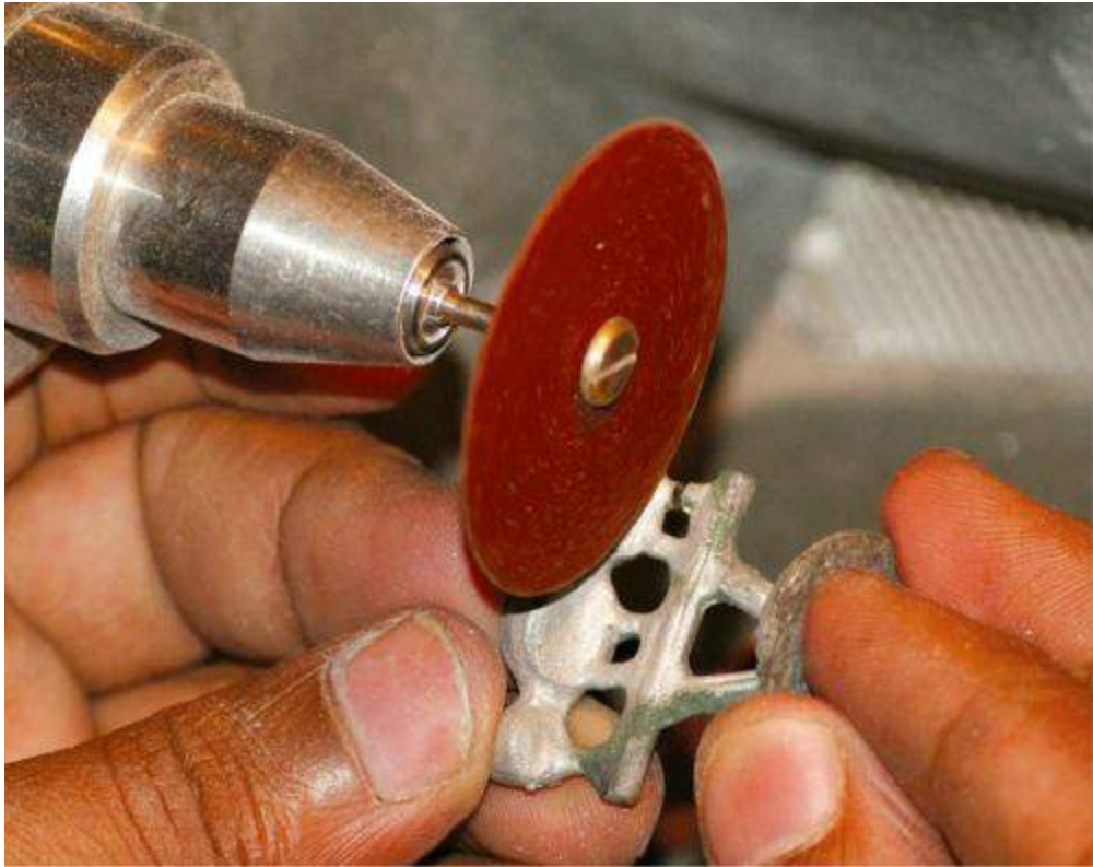
FIGURE 40.81 The sprue is separated from the casting using a carborundum disc.
