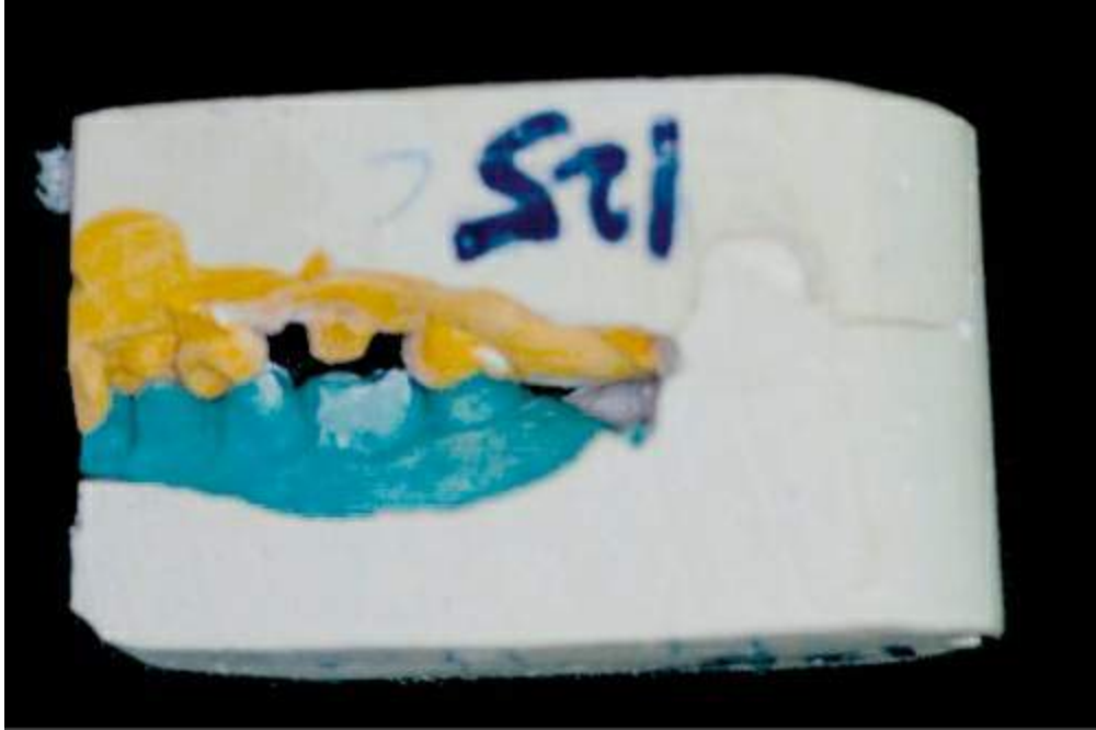
FIGURE 37.33 Index used as a hinge articulator.
