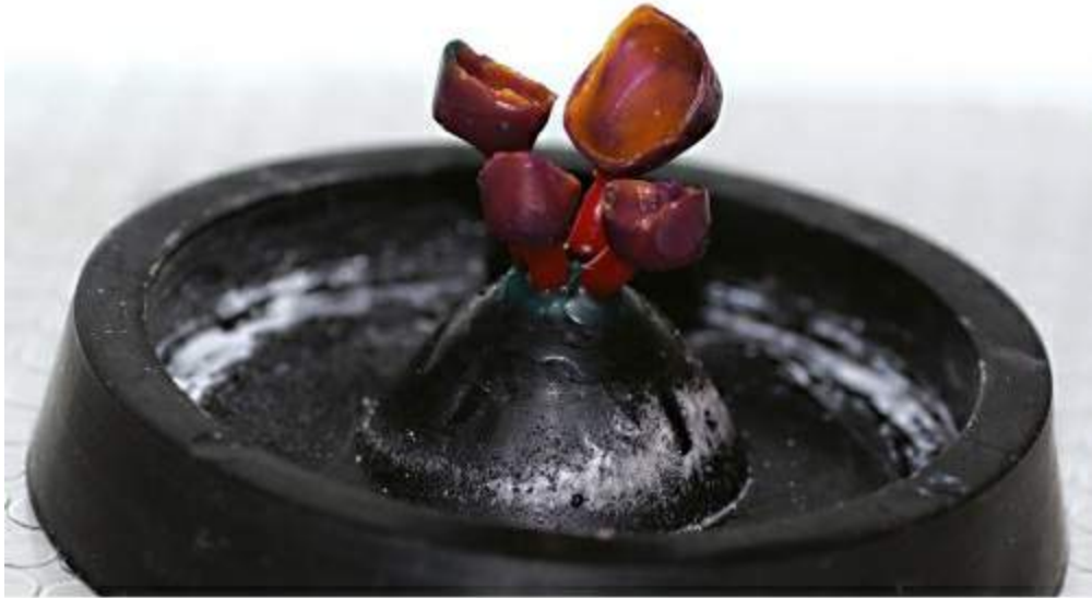
FIGURE 40.60 Sprue former attached to the conical part of sprue former, which after investing and burnout forms the entry to the mould space.
