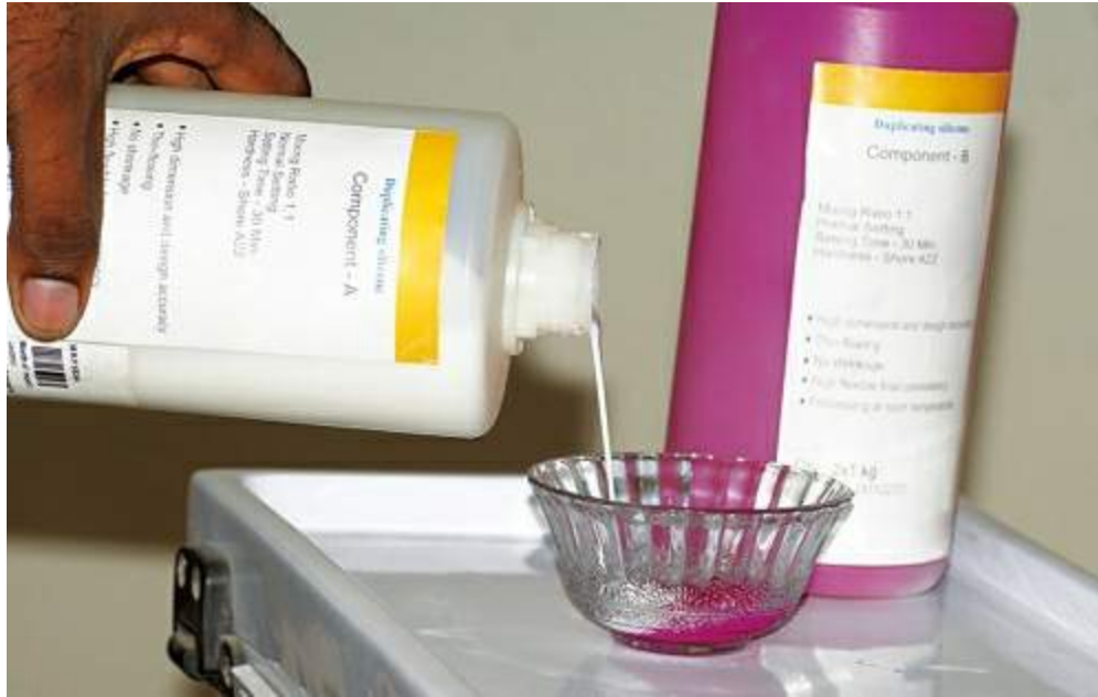
FIGURE 27.2 Silicone duplicating base material (pink) is mixed with the catalyst (white) in equal amount in a clean bowl and mixed.
