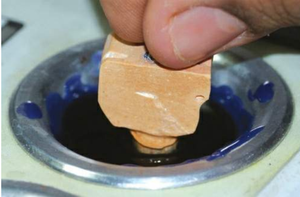
FIGURE 40.25 Die dipped in molten wax.
