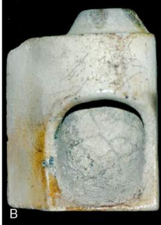
FIGURE 40.69 Quartz crucible used for (A) induction casting and (B) centrifugal casting.
