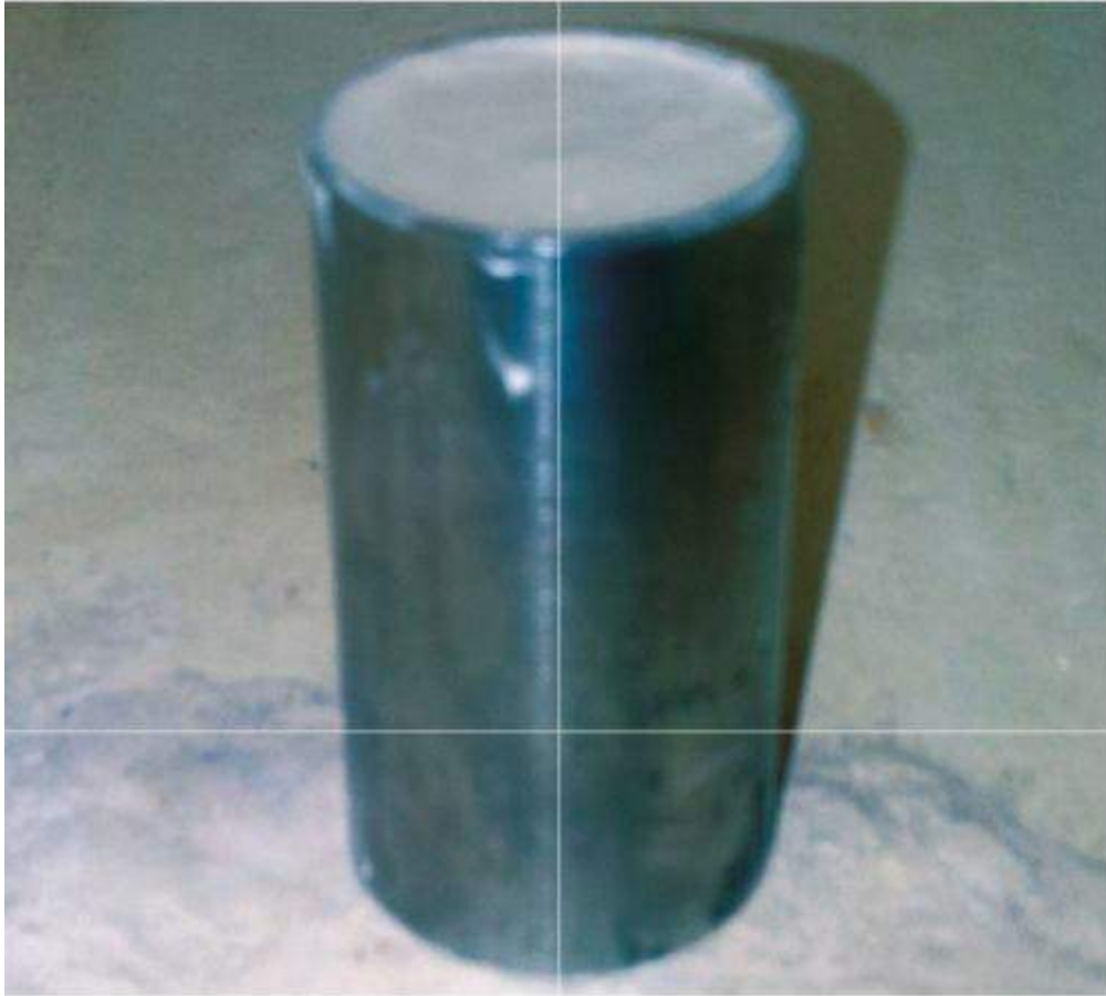
FIGURE 40.68 The ring should be placed with the sprue hole facing down.
