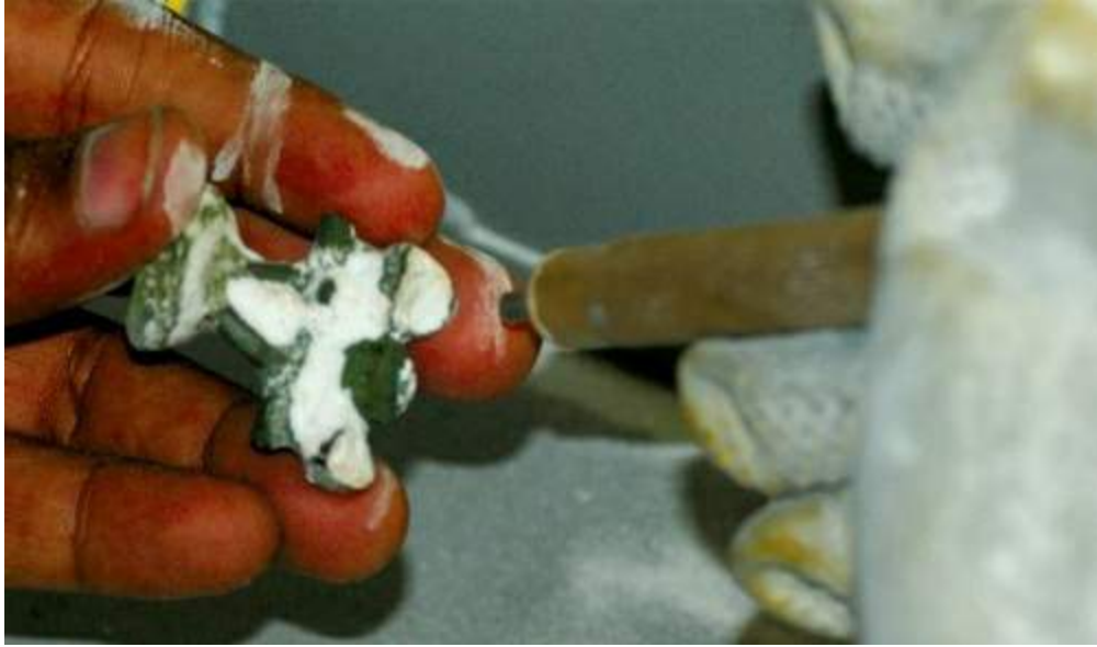
FIGURE 40.78 The investment material is removed by sandblasting.
