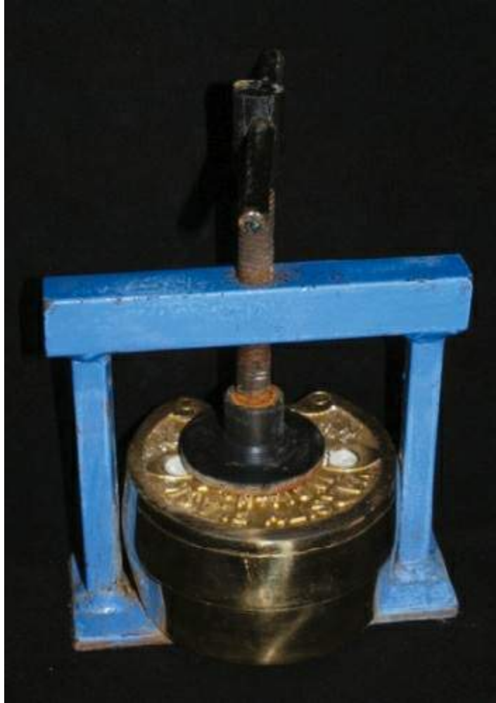
FIGURE 12.13 Flask tightened with clamp.
