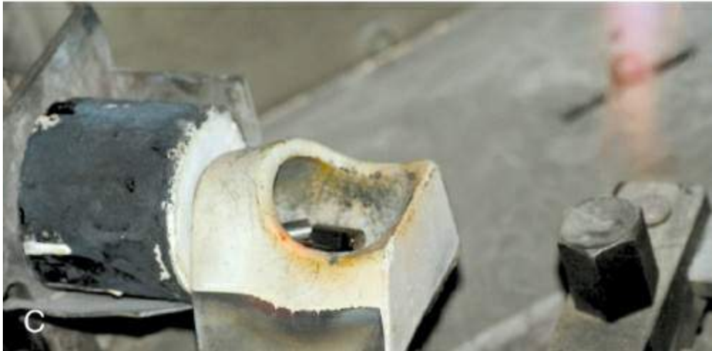
FIGURE 40.74 (A) The casting ring is removed from the furnace. (B) The casting ring is placed in the cradle of the casting machine. (C) The crucible containing metal pellets directed towards the mould space created by the conical crucible former.
