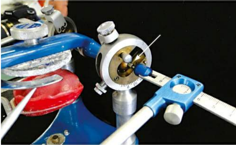
FIGURE 6.25 Facebow is mounted by placing the condylar rods at the centre of the condyle in the articulator.
