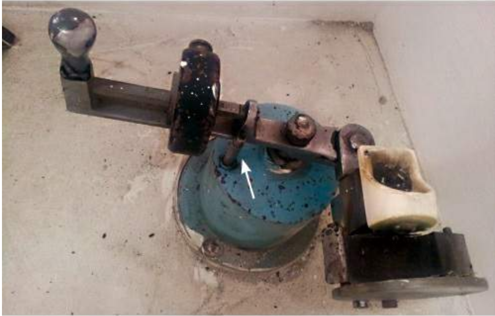
FIGURE 40.71 The arm of the machine is given three turns and locked with the pin.
