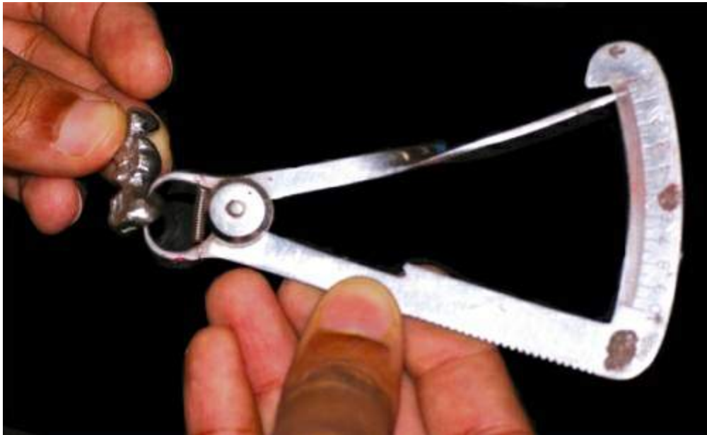
FIGURE 40.86 The metal caliper is used to check the thickness.
