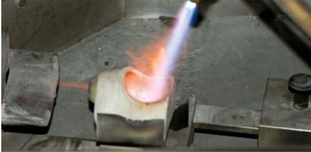
FIGURE 40.73 The crucible is preheated with the flame.
