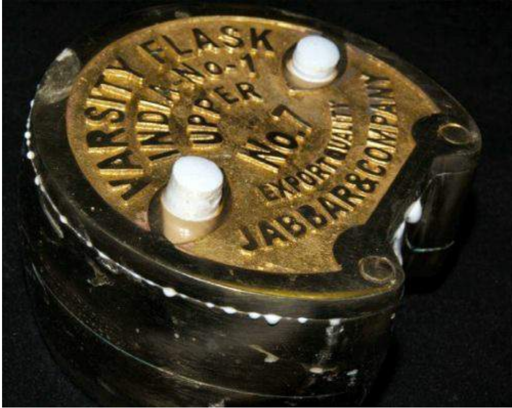
FIGURE 12.12 Excess plaster escaping through lid.
