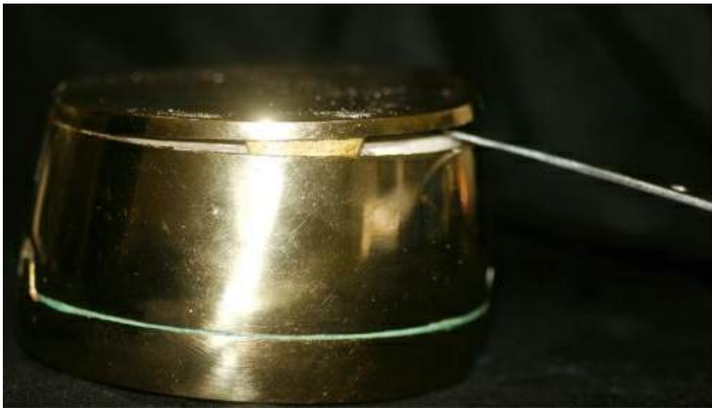
FIGURE 12.24 The lid is removed by prying with wax knife.
