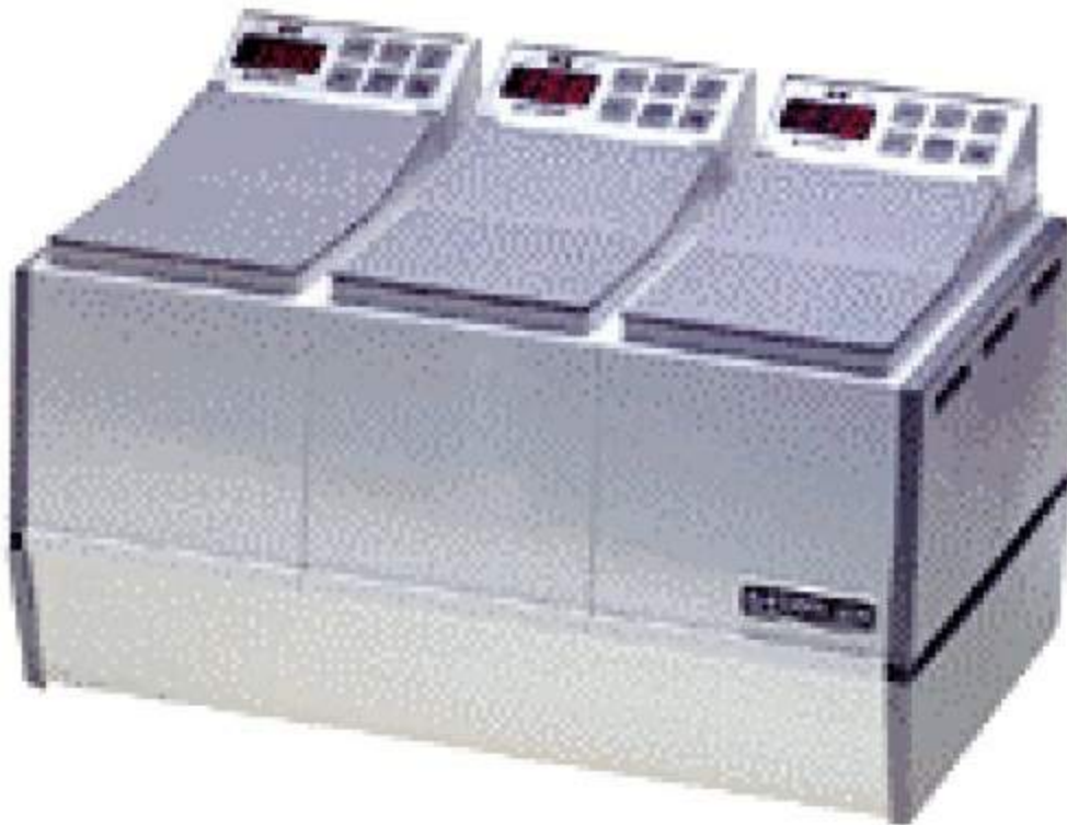
FIGURE 37.1 Equipment for agar with liquefying, storage and tempering baths.
