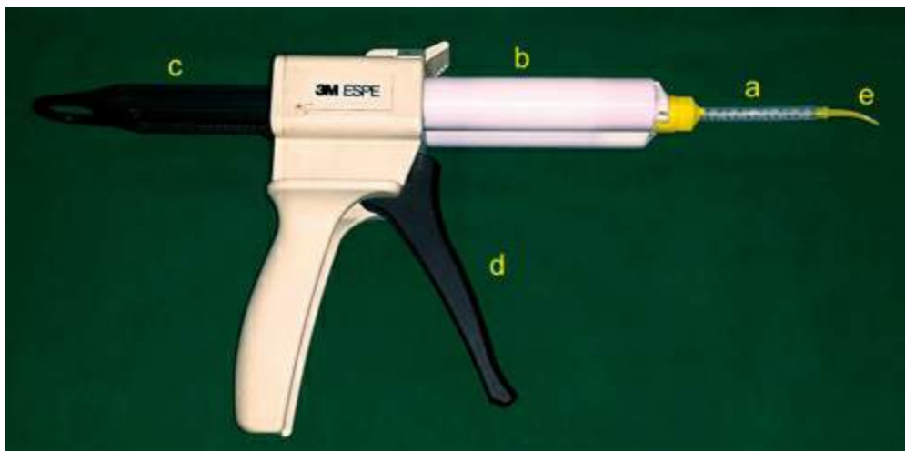
FIGURE 37.6 Anautomix gun with material: spiral mixing tip (a), cartridge containing base and catalyst (b), plunger (c), trigger (d), intraoral tip (e).
