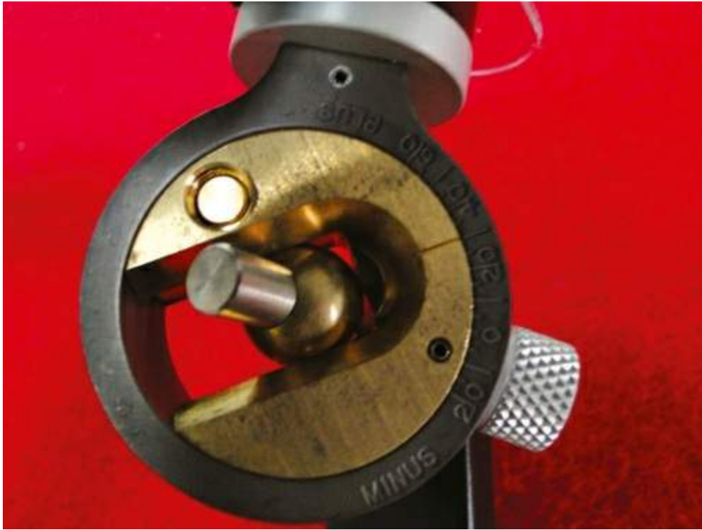
FIGURE 33.15 Horizontal condylar inclination is set at 30°.
