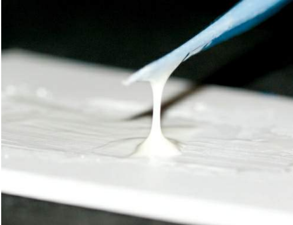
FIGURE 41.26 Cement that is ready to use will string out from the lifted spatula.
