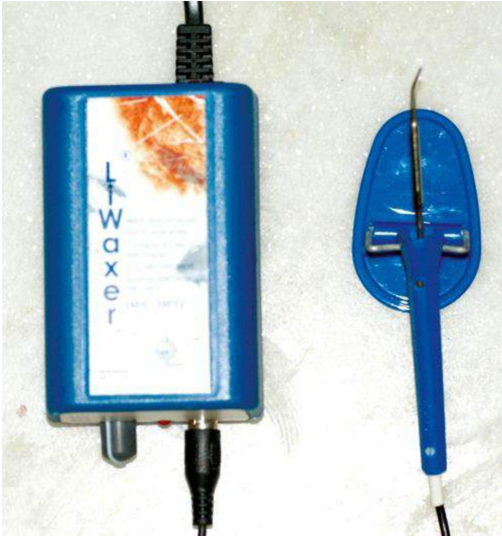
FIGURE 40.22 Electric waxing unit.
