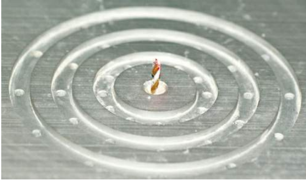
FIGURE 40.16 Pindex machine platform. Drill in the platform makes a hole on the base of cast whereas indicated by the laser pointer.
