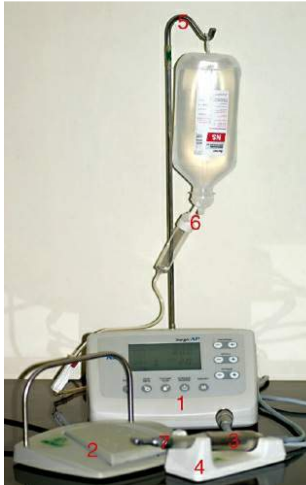
FIGURE 49.81 Parts of a typical physiodispenser 1. Display & controls 2. Foot pedal 3. Micromotor 4. Handpiece stand 5. Stand for normal saline 6. Irrigation set 7. Reduction gear handpiece.
