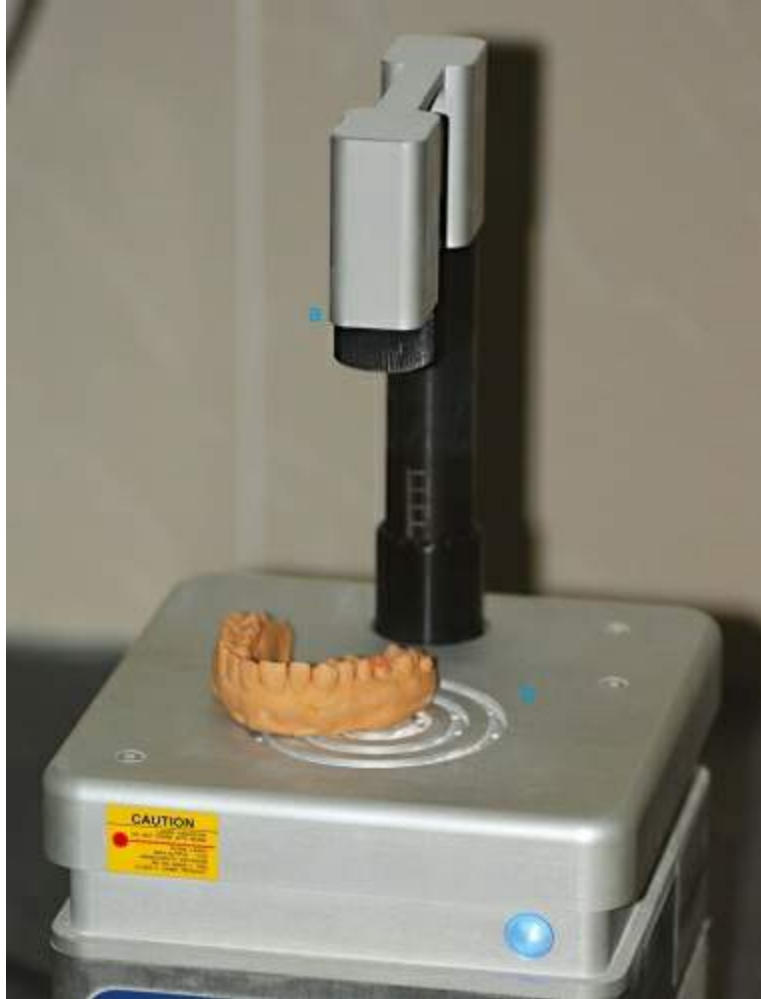
FIGURE 40.15 Pindex machine: laser pointer (a), platform (b).
