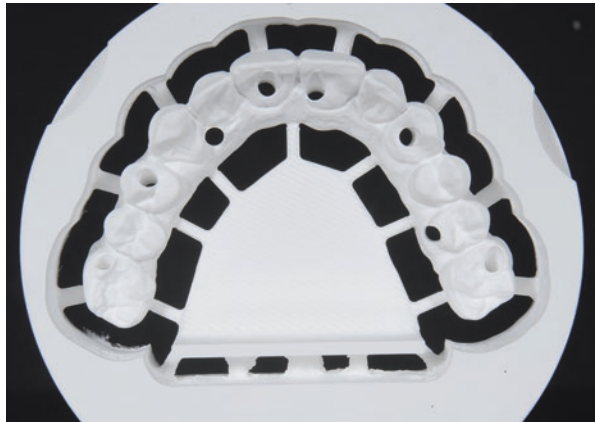
Fig. 9.69 Full zirconia prosthesis prepared with special milling burs
