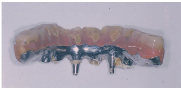
Fig. 14.48 Multiple fatigue fractures of older generation, externally threaded Diskimplants® after 11 years of function
