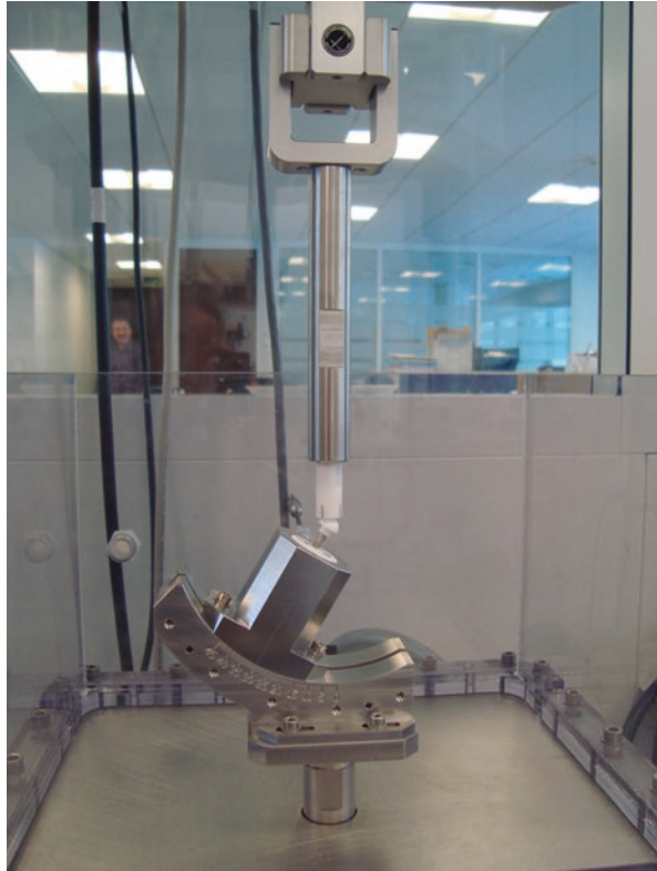
Fig. 3.2 Fatigue testing machine for dental implants (courtesy Hervé Richard, Anthogyr)
