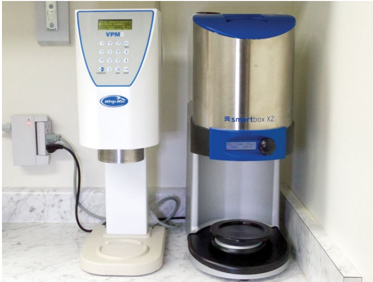
Figure 3.27 Automatic dispensing unit and automatic vacuum mixing unit for dental stone.
