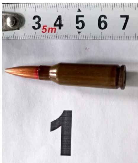
Fig. 1. General appearance of the cartridge: 1 – 5.45x39 mm a cartridge with “PS” bullets with a steel core.
