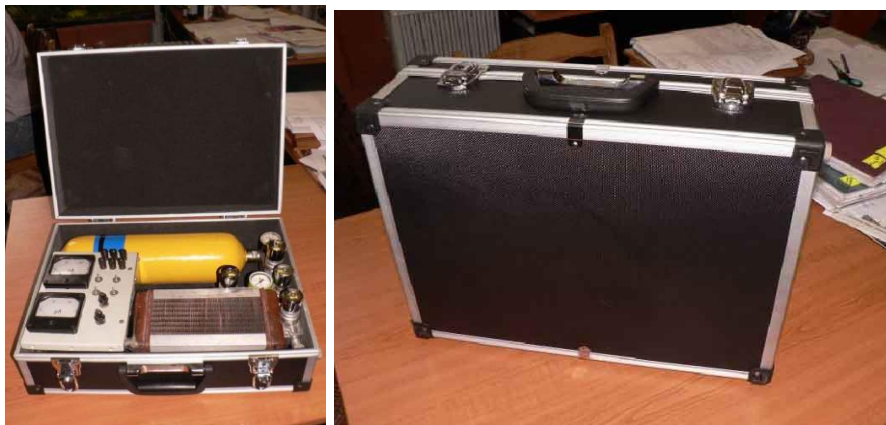
Figure. 4. A working sample of a metal hydride power source for exploitation of equipment in the field.
