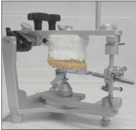
Fig. 2-45. Mounting the upper jaw cast in articulator with face-bow assembly (bite fork and fixating device). (Whip-Mix USA)
