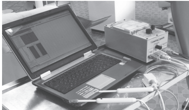
Fig. 1. An apparatus for measuring electric power characteristics in the oral cavity ("CompaDent")
