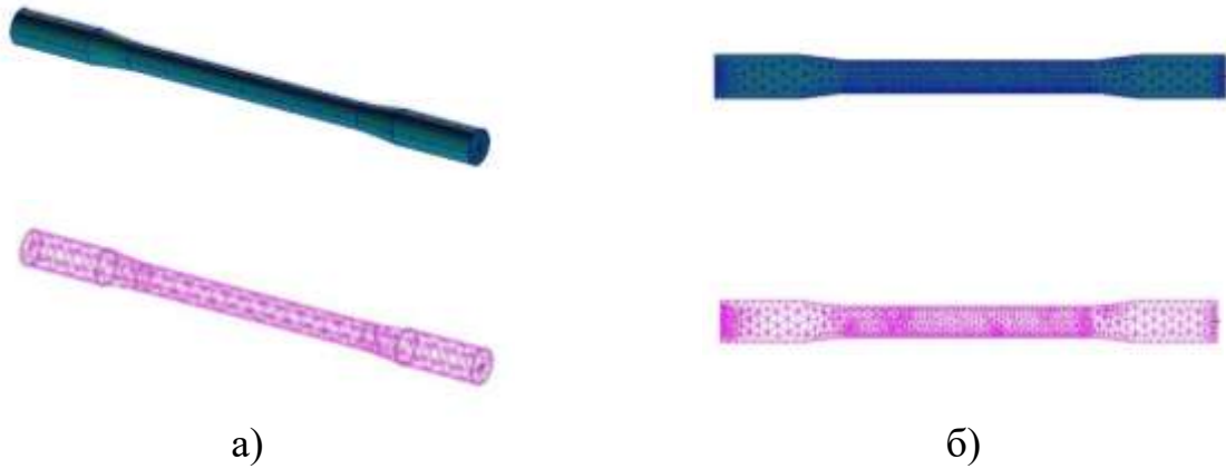
a) b) Figure 3. Samples divided into a finite element grid: a – SLM, b – GPDLG.
