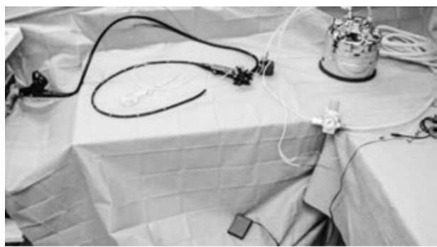
Figure 8. Waterjet necrosectomy device, prototype [93]
