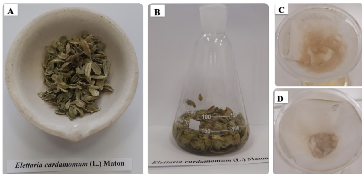
Figure 1. Stages of the study: A – prepared raw materials for weighing, B – pericarp before extraction, C – filtered precipitate ready for complete drying, D – dried precipitate.
