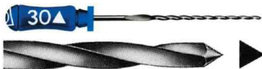
Fig. 8.9. K-reamer: general view, working part shape and symbol
