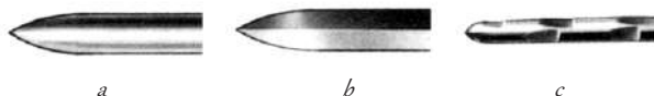
Fig. 8.4. Smooth broashes: a – with a round cross-section, b – broashes of Miller (faceted), c – broashes for fixing of turundas
