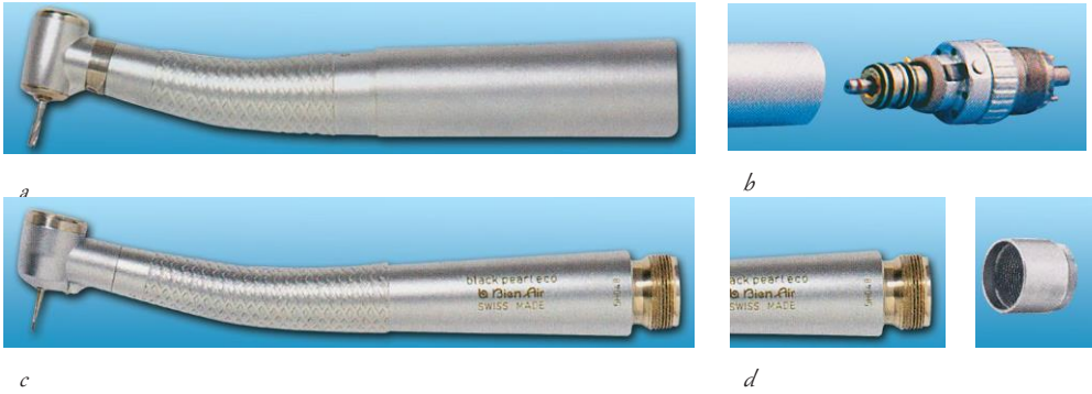
Fig. 1.9. Types of fixing the high-speed (turbine) handpiece: a – turbine handpiece on air bearings, rotation speed up to 450 000 rpm. Fixing the handpiece with Unifix type of connector; b – quick-detachable connector of Unifix type; c – turbine handpiece on metal bearings, speed of rotation up to 310 000 rpm; d – fixing system of the handpiece – direct hose connection with screw
