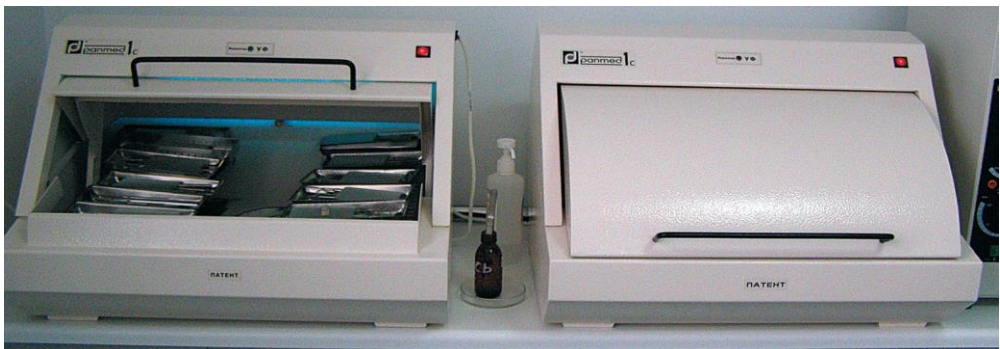
Fig. 2.8. Ultraviolet chambers for storage of sterile instruments
