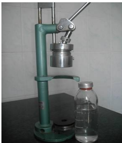
Fig. 39. The rolling machine
